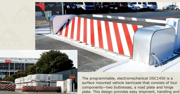
installation. The barrier components are lag-bolted in place to existing concrete surfaces such as parking structures and parking lots to be used as an anti-theft and/or traffic control device. The barricade features a self-contained programmable electromechanical drive system, controls and an integral barrier arm. Typical installation is four hours or less.
